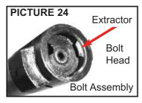
Air dry or use compressed air to thoroughly dry all components in the bolt assembly.
