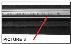
**WARNING!** Only use the specified cartridge type and caliber of projectile specified for your firearm as designated on the barrel. Use of an improper caliber or ignition component in your firearm could result in property damage, personal injury and/or death.
