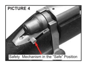
Always engage the safety mechanism by moving the safety lever fully rearward before handling, loading or unloading the firearm.
