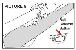
6. Push the bolt assembly forward until the bolt stop is engaged, and the bolt assembly is locked into the receiver.
