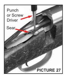
**WARNING!** If the sear does not return to the full upward position without hesitation, then your firearm is **NOT** in a safe operating condition and must **NOT** be used until you have it inspected and the problem corrected by a Remington Authorized Repair Center. Discharging a firearm which does not function properly may lead to property damage, personal injury and/or death.
